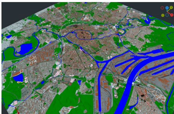
Figure 5. Mesh of Strasbourg, containing elevation, green areas, roads, water bodies and buildings. Visualized using Ktirio GUI.
