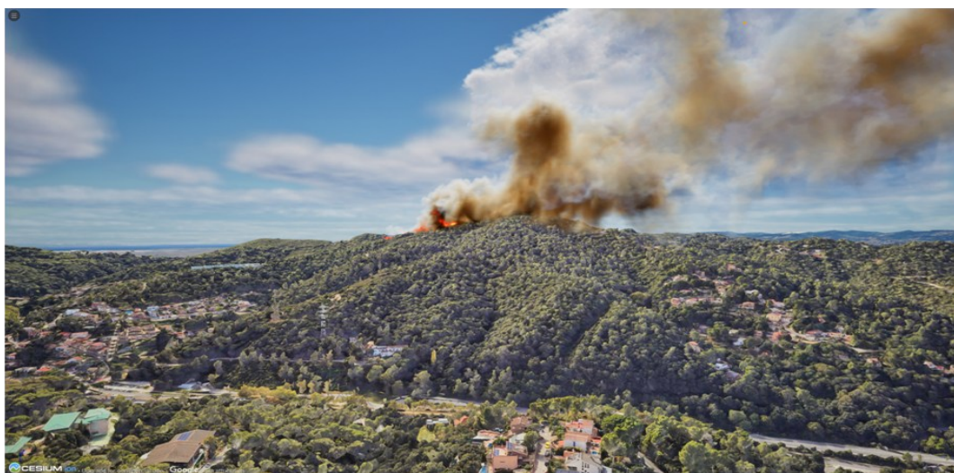
Figure 3. Example of the integration of a flame front and smoke column simulation onto the geometry provided by CESIUM from the Google Tile Service.
