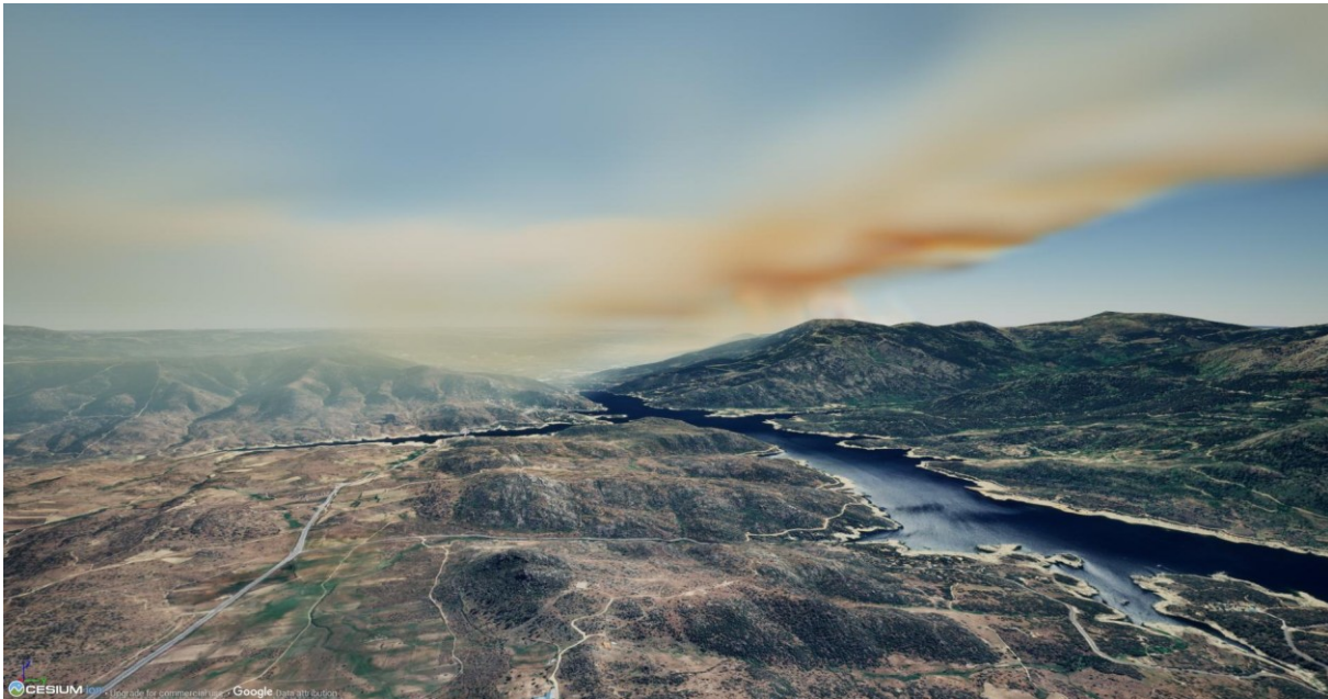
Figure 15. Figure 16. The same simulation, but viewed closer to the ground. The orange tint caused by Mie scattering due to the presence of particles in the atmosphere is clearly visible.
