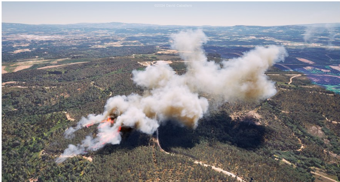
Figure 2. Effect of smoke shadow projection on the terrain, in this case provided by the CESIUM service. The shadow density is proportional to the attenuation of light as it passes through the volume defined by the smoke column. The effects of Rayleigh scattering.
