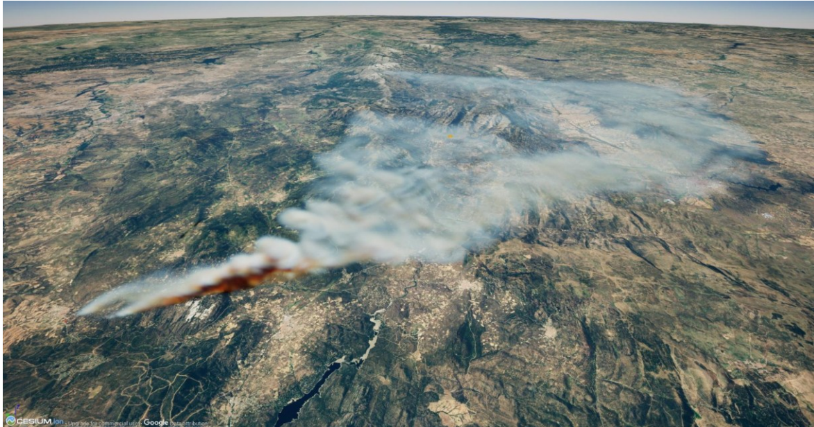
Figure 14. Example of integrating WRF-SFIRE simulations into Unreal Engine 5 using Google Tile Service geometry via CESIUM for the 2019 Cadalso de los Vidrios wildfire.
