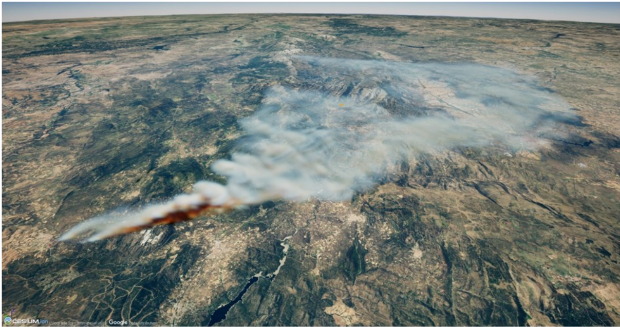
Figure 3 Example of integrating a CFD simulation done in WRF-SFIRE of volumetric smoke and fire from a wildfire into a photo-realistic immersive environment using Unreal Engine. The digital terrain model has been replaced by the Cesium-Google Tiles service. Some vector GIS layers and background volumetric clouds have been added.
