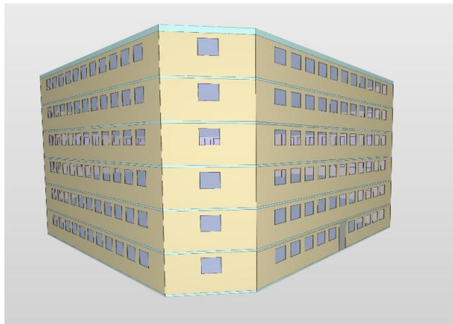
Figure 3 Windows and doors on a generated building IFC, viewed using Solibri.
